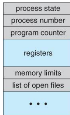
Figure 2.16 - Process control block (PCB)
